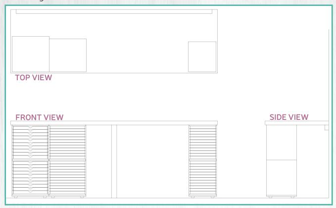
The Alex drawer can replace both front and rear support legs on most table tops that are about two feet deep.
